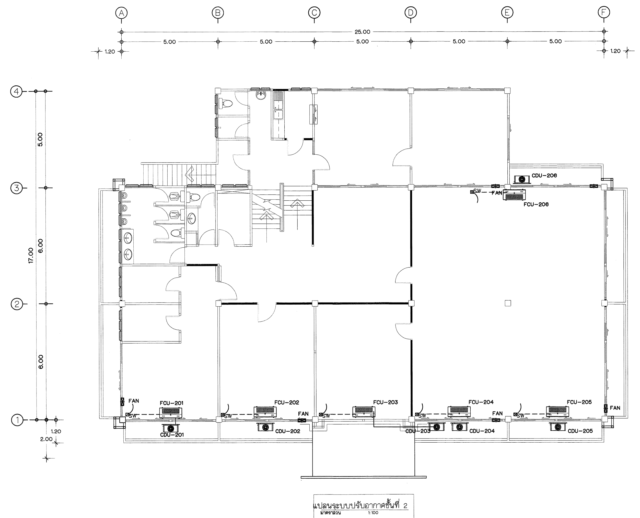
เครื่องยี่ห้อ SUPPLY AIR QUANTITY (CFM) TOTAL CAPACITY ไม่น้อยกว่า BTU/HR TYPE OF FANCOIL UNIT COMPRESSOR POWER SUPPLY VENTILATING FAN (in) NO.101 18,000 / CEILING MOUNTED 220/1/50 8" NO.102 18,000 / CEILING MOUNTED 220/1/50 8" NO.103 18,000 / CEILING MOUNTED 220/1/50 8" NO.104 24,000 / CEILING MOUNTED 220/1/50 8" NO.105 24,000 / CEILING MOUNTED 220/1/50 8" NO.106 12,000 / WALL MOUNTED 220/1/50 8" NO.107 12,000 / WALL MOUNTED 220/1/50 8" NO.201 24,000 / CEILING MOUNTED 220/1/50 8" NO.202 24,000 / CEILING MOUNTED 220/1/50 8" NO.203 24,000 / CEILING MOUNTED 220/1/50 8" NO.204 36,000 / CEILING MOUNTED 220/1/50 8" NO.205 36,000 / CEILING MOUNTED 220/1/50 8" NO.206 36,000 / CEILING MOUNTED 220/1/50 8" NO.301 12,000 / WALL MOUNTED 220/1/50 8" NO.302 24,000 / CEILING MOUNTED 220/1/50 8" NO.303 36,000 / CEILING MOUNTED 220/1/50 8" NO.304 36,000 / CEILING MOUNTED 220/1/50 8" NO.305 30,000 / CEILING MOUNTED 220/1/50 8" NO.306 30,000 / CEILING MOUNTED 220/1/50 8" NO.307 30,000 / CEILING MOUNTED 220/1/50 8" NO.308 18,000 / CEILING MOUNTED 220/1/50 8" NO.309 18,000 / CEILING MOUNTED 220/1/50 8"
